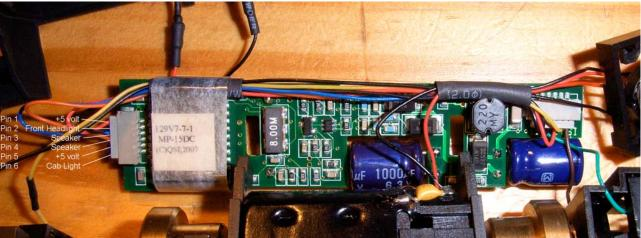
The first picture shows the top of the circuit board, what you see when you open the shell. The Rear Headlight is wired to the two pads at the left corners of the board.
