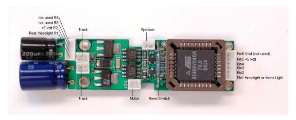
The pins labeled Pin1, Pin2, Pin3, and Pin4 in the connector to the right of the flash memory chip are used for lights. Pin5 is +5 volts and is the return for Pin1, Pin2, Pin3, and Pin4 lights.
