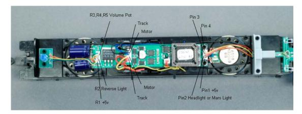
The picture shows the board installed in a LifeLike E8. In this model there is no reverse light connected to R2.
