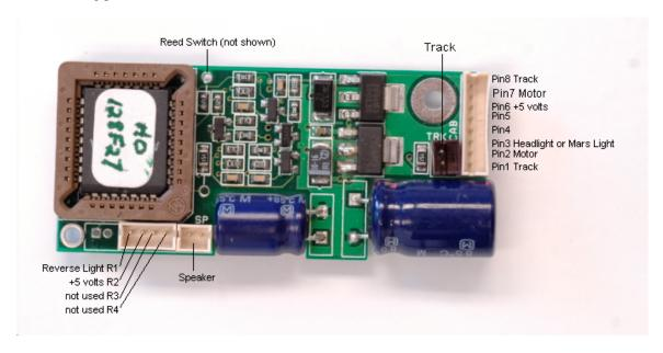
The pins labeled Pin3, Pin4, and Pin5 in connector at the right of this picture are used for lights. Pin6 is +5 volts and is the return for Pin3, Pin4, and Pin5 lights.
